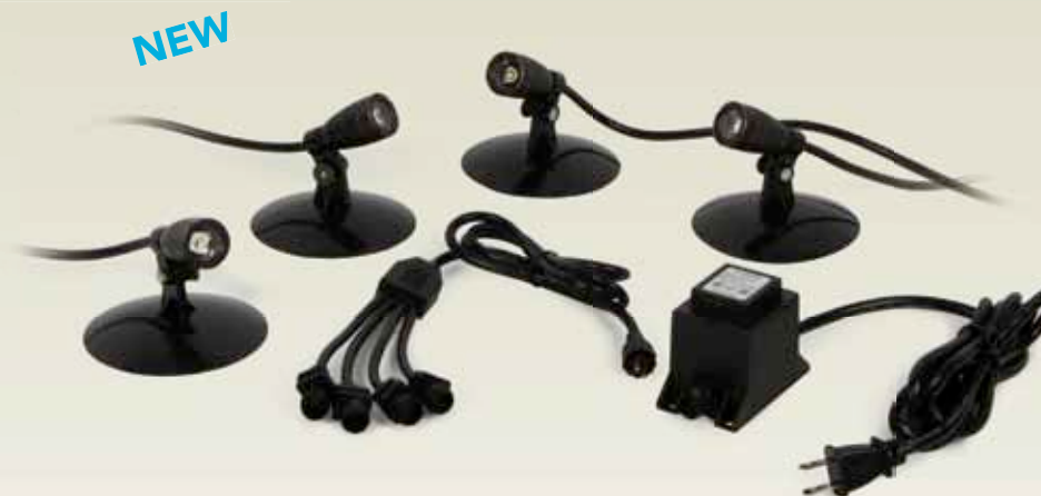
Model: SOLW2X4 Description: 4 pack / Compact Spotlights Input Voltage: 12 volt AC Watts: 8 Beam Angle: 45 Degrees Includes: (4) SOLW2 Compact Spotlights, transformer and 4-way splitter
