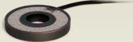
Model: SOLWLR Description: Warm White Light Ring Input Voltage: 12 volt AC Watts: 7 Beam Angle: 150 Degrees Dimensions: 3½"OD x 1⅜"ID x ¾"H Includes: LED Light Ring, 20' power cord w/ quick-connect plug
