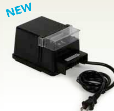
Model: SOLTRANS88 Description: 88 Watt Transformer Input Voltage: 120 volt AC Output Voltage: 12 volt AC / 88 watts Dimensions: 4" L x 4" W x 7" H
